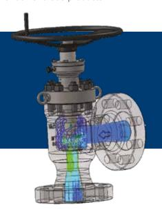
Our R&D technicians and engineering team make use of an advanced internal software for valve sizing, based on ISA S75.01 formulae and SolidWorks Flow Simulation to verify valve components and their functioning.
